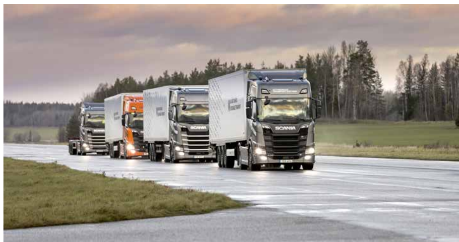
The haulier Ahola will use Scania trucks in real-traffic conditions to test semi-autonomous platooning formations with three or more connected trucks.
